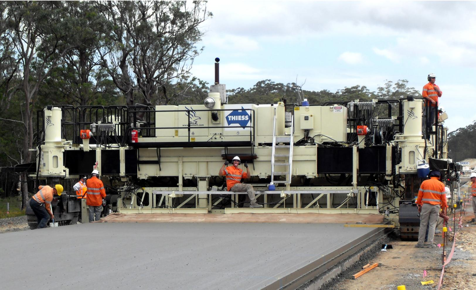
The S1500 Slipform Paver is the largest paver offered by G&Z. Its stout design makes it capable of meeting the strictest smoothness specifications at wide multiple-lane paving applications. The S1500 features a telescopic tractor frame, telescopic front walkway, and a hose tray that can telescope from 18' (5.5m) to 42' (12.8m), the largest in the industry. Its time tested and proven design makes the S1500 the paver of choice for multiple-lane mainline and airport work.
