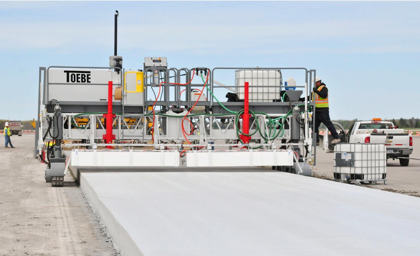
The G&Z TC1500 is the most technologically advanced texture cure machine on the concrete paving market today. The features contributing to this best-in-class distinction include the four-track 90 degree capabilities, the highly accurate steering and elevation control systems, and unique frame design for quick width changes.
